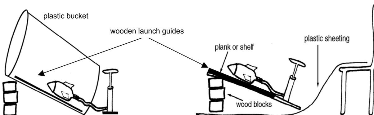
Two possible launch systems. The one with the bucket is safer and creates less mess.
